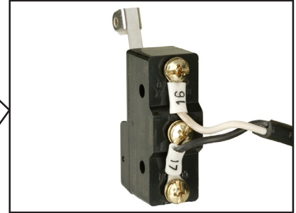
Figure 69. Limit switch wiring.
